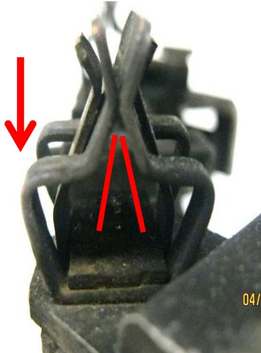
Jaws are bent and do not meet parallel in the center.
